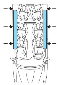
The Safety Canopy System, in combination with safety belts, can help reduce the risk of severe injuries in the event of a significant side impact collision or rollover event.
